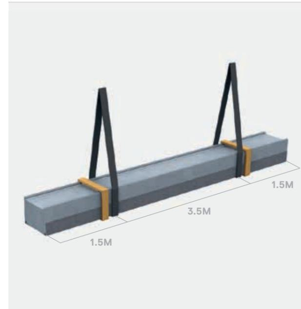
When using a lifting beam to lay the packs of panels on a curved roof surface, use belts of sufficient lengths to avoid the lifting beam coming into contact with the roof surface before completely setting down the packs.
