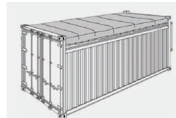
Open Top 20' – Inner dimensions: L=5895mm W=2350mm H=2380mm
