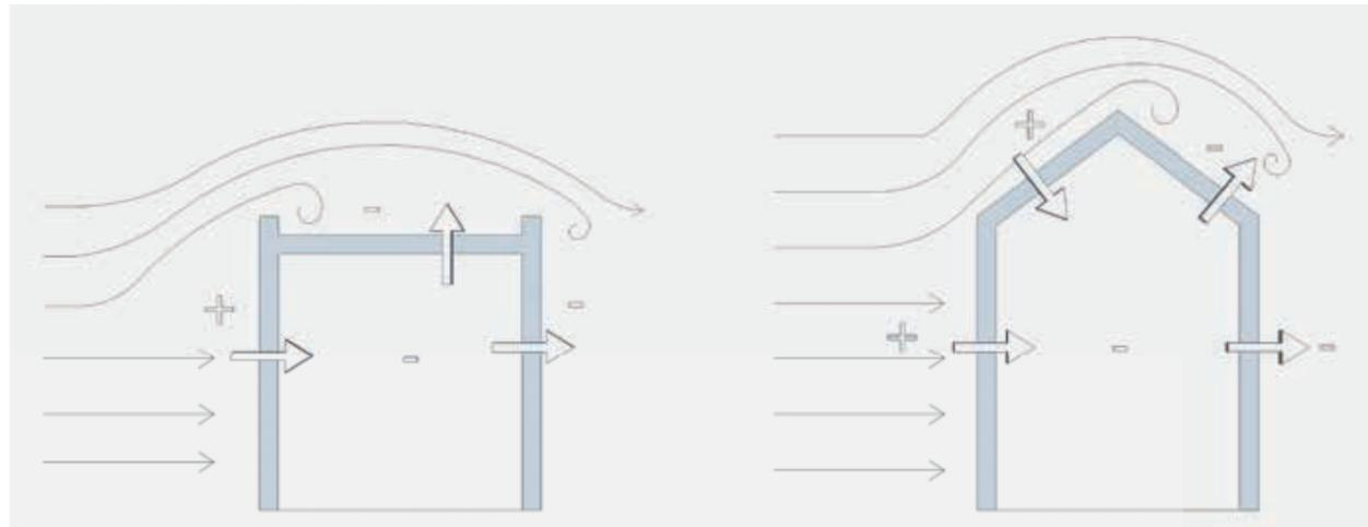
FIGURE 2: ROOF WIND LOADS – CRITICAL ZONES
