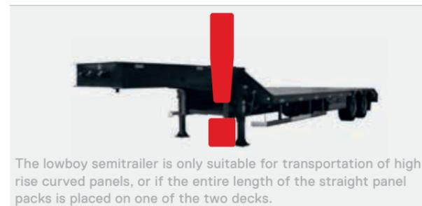
The lowboy semitrailer is only suitable for transportation of high rise curved panels, or if the entire length of the straight panel packs is placed on one of the two decks.
