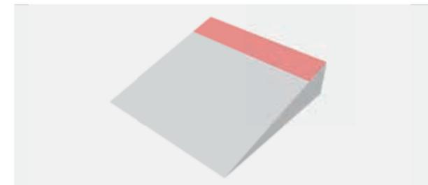
In the above image, the fixed-point area should be located in the same position for all panels. More than one fixed-point area per panel length should be avoided to prevent the buckling of panels, shearing of fixings or opening of seams.
