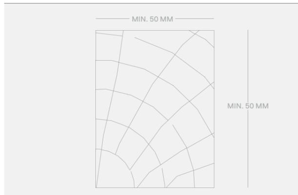
All wood types used in construction are allowed, so long as the mechanical strength and dimensional stability are checked. Strength class (EN338)  $\geq$  C24,  $\rho = 350\text{kg/m}^3$ . When delivered, the wood humidity must be slightly lower – in any case not higher than 18% - than the humidity of the place where it will be stored and used. This may be achieved by natural or artificial aging.
