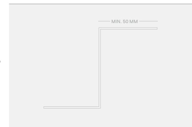
The metal support elements are generally cold shaped profiles (C, U, Z, Ω sections) made from galvanized steel.
